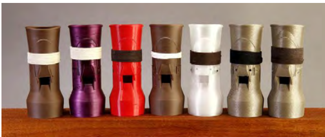
Seven headjoints fabricated from several types of PLA and Copolyester filaments
